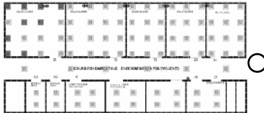
Fig. 10. Measured service coverage for Business service (user throughput threshold = 2 Mbit/s, 94 locations): the light grey squares are the locations where the service coverage is acceptable; the dark grey squares are the location where the service coverage is below threshold. The access point is located at the center of the circle.
