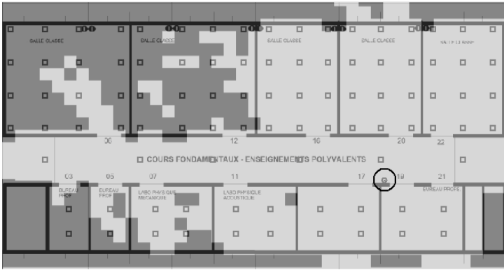
Fig. 15. Predicted “Interactive service” coverage in light grey. The access point is at the center of the black circle. The PixelFlow parameters are as in Fig. 13.
