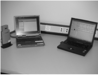
Fig. 7. The measurement equipments set-up used to conduct the measurements: the WLAN access point on the left is linked to the leftmost PC via a cross-over Ethernet cable. The right most PC is the client with our own survey software.
